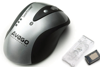
Figure 3: ADNS-7633 mouse design kit
